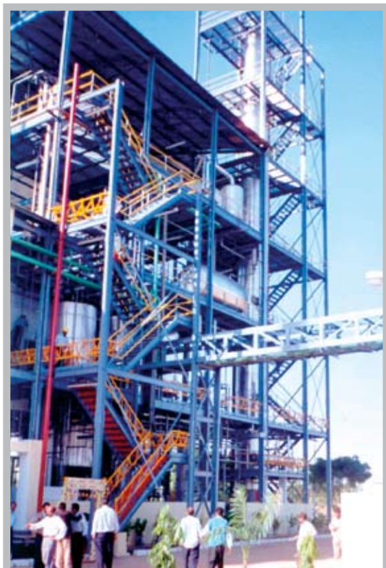
“UNITOWER” continuous fats splitting plant Capacity: 120 t/d
