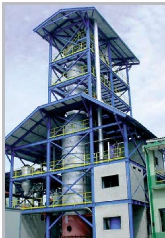
Deodorization/deacidification plant (Colombia) - Capacity: 500 t/d
