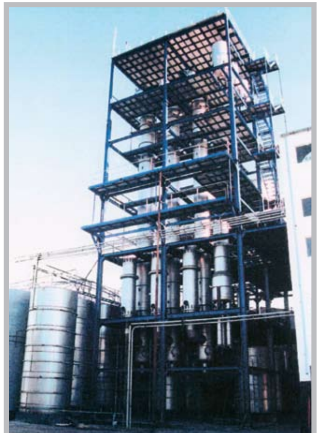
Fatty acids distillative fractionation plant Capacity: 180 t/d
